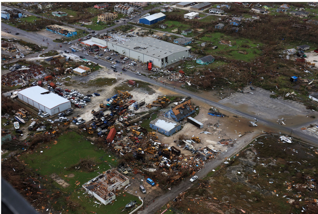
Figure 4.7. Aerial photo of the damage from Dorian at Marsh Harbour on Great Abaco Island, Bahamas. Note the surviving commercial and industrial buildings with minor roof damage. [The large building in the center is located at 26.532695 / -77.062676]. The photo was taken facing SW. (Source: CNN )
