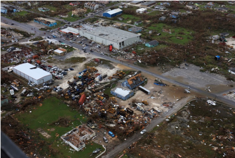
Photo from the main report— Figure 4.7. Aerial photo of the damage from Dorian at Marsh Harbour on Great Abaco Island, Bahamas. Note the surviving commercial and industrial buildings with minor roof damage. [The large building in the center is located at 26.532695 / - 77.062676]. The photo was taken facing SW. (Source: CNN )
