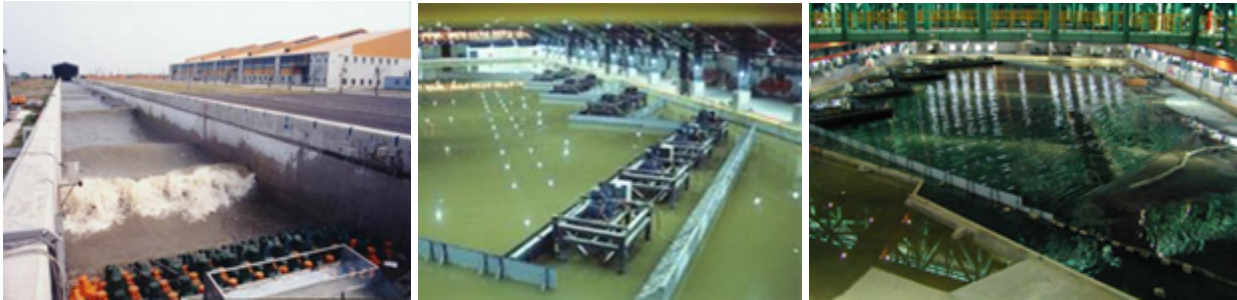
Fig. 1 research facilities of THL (a) Long wave flume, 300m X 5m X 5.2m (b,c) Near Shore Basin (150m X 60m)
