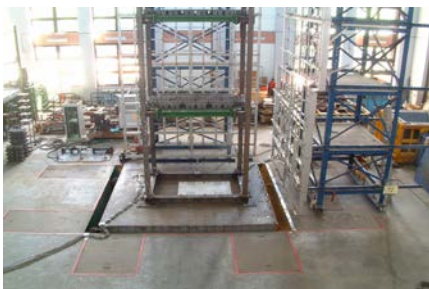
3D earthquake simulator (5mx5m)
