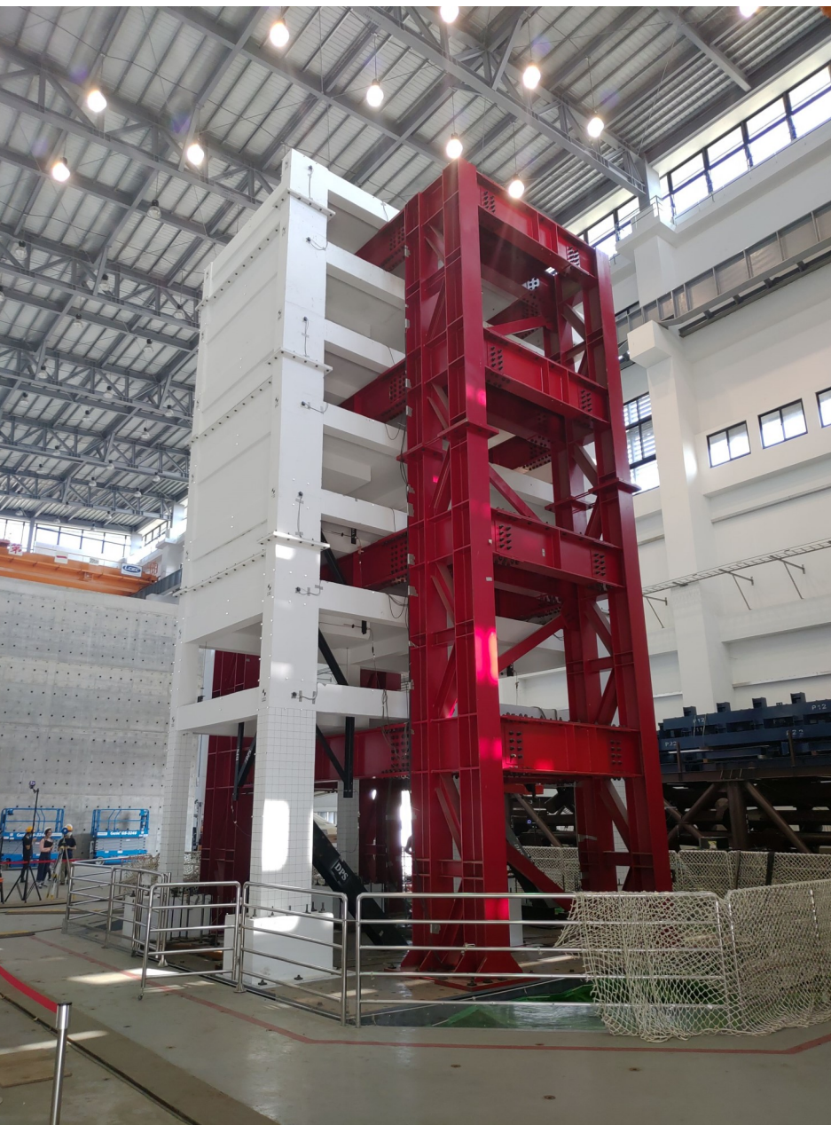
Fig.1. The shaking table test on soft- and weak-story building
