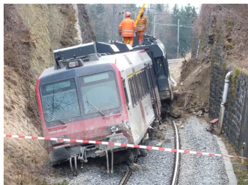
Train derailed in February 2013 (Switzerland), because of a wall failure caused by heavy rainfall, demonstrating the effect of aging of infrastructures.
