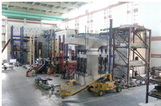
L-shape reaction wall and strong floor
