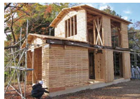
Experimenting seismic reinforcements of column-walls in a real size wooden house
