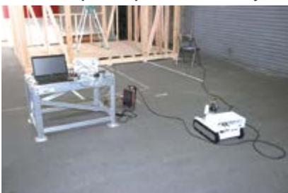
This robotic system estimates the strength of beams in a burnt structure from a remote position and helps firefighters to make decisions of safe entry into the burnt area.
