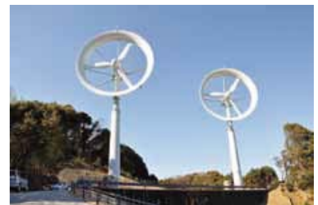
100kW Wind-lens turbine
