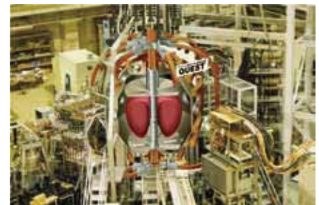
Kyushu(Q-shu) university experiment with steady state spherical tokamak (QUEST) to research fundamentals for a steady state operation of future fusion power plants
