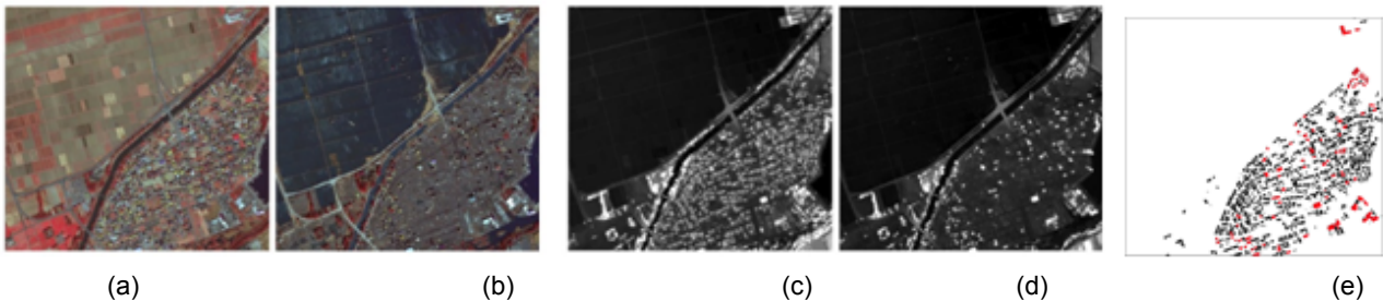
Figure (a) and (b) show the false color pan-sharpened pre- and post-earthquake GeoEye-1 image, with 0.5 m spatial resolution, respectively. Figure (c) and (d) show the pre- and post-earthquake digital surface model (DSM) image, with 0.5 m spatial resolution, respectively. Figure (e) shows the detection result by the ND-method. The black areas signify the destroyed buildings, and the red areas the survived buildings.
