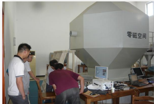
Magnetic field-free space for calibrating instruments
