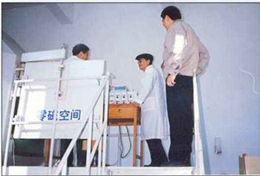
Magnetic field-free space for calibrating instruments
